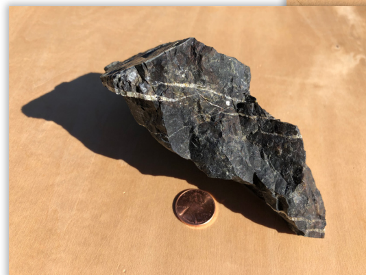
Left: Veinlets of chrysotile asbestos in partially serpentinized ultramafic rock. When properly oriented in sunlight, the veinlets exhibit silky luster and cross-fiber texture. Penny for scale. Photo: Chris Higgins, CGS.
