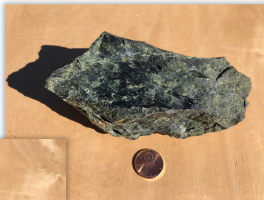
Right: Serpentinite with typical mottled grayish-green color and greasy luster. The luster results from intense shearing of the rock. Penny for scale. Photo: Chris Higgins, CGS.
