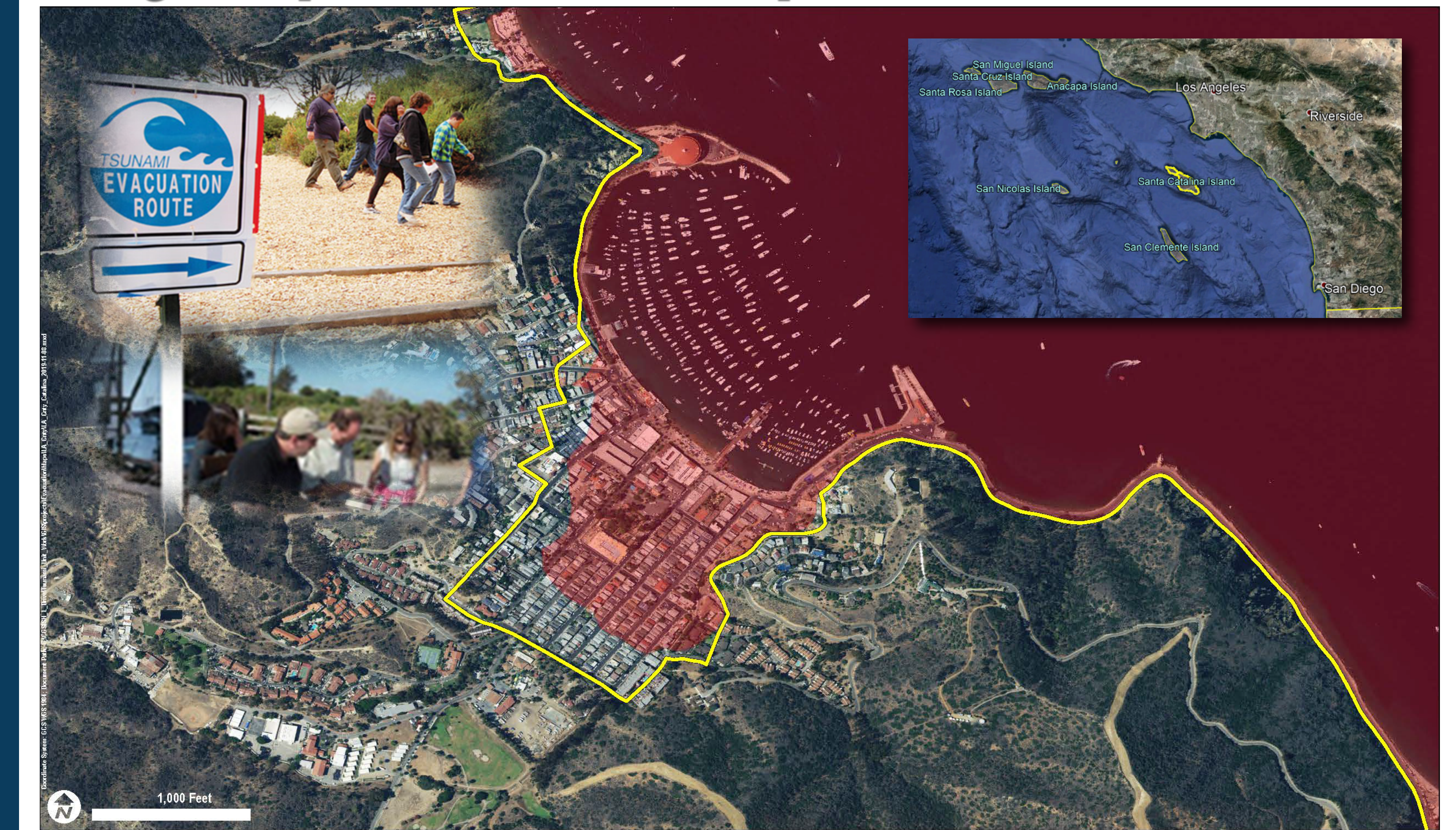
Map of Avalon on Santa Catalina Island, California showing the inundation and draft evacuation line for locals to review. The updated inundation area is based on science (i.e., tsunami modeling), whereas the evacuation line is typically drawn further inland to an easily identifiable geographic feature, such as a road. However, each local agency ultimately determines where their evacuation line will be drawn based on their emergency response needs.
