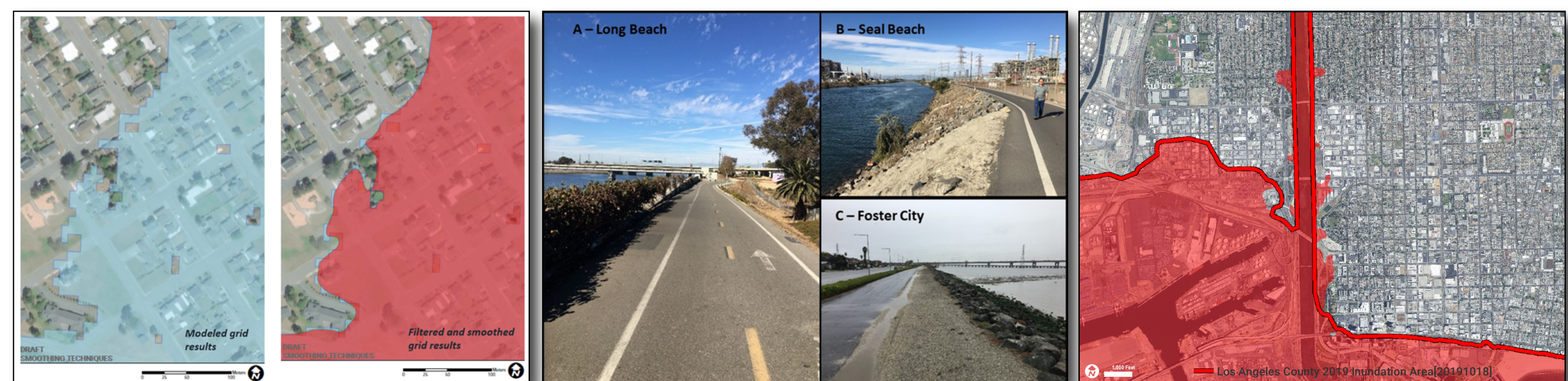
Comparing unprocessed PTHA results (blue blocky area) to the post-processed results (red filtered and smoothed area). Post-processed results on the right are prepared using a semi-automated filtering process that removed holidays and applied a smoothing algorithm to create a more realistic looking inundation boundary.
