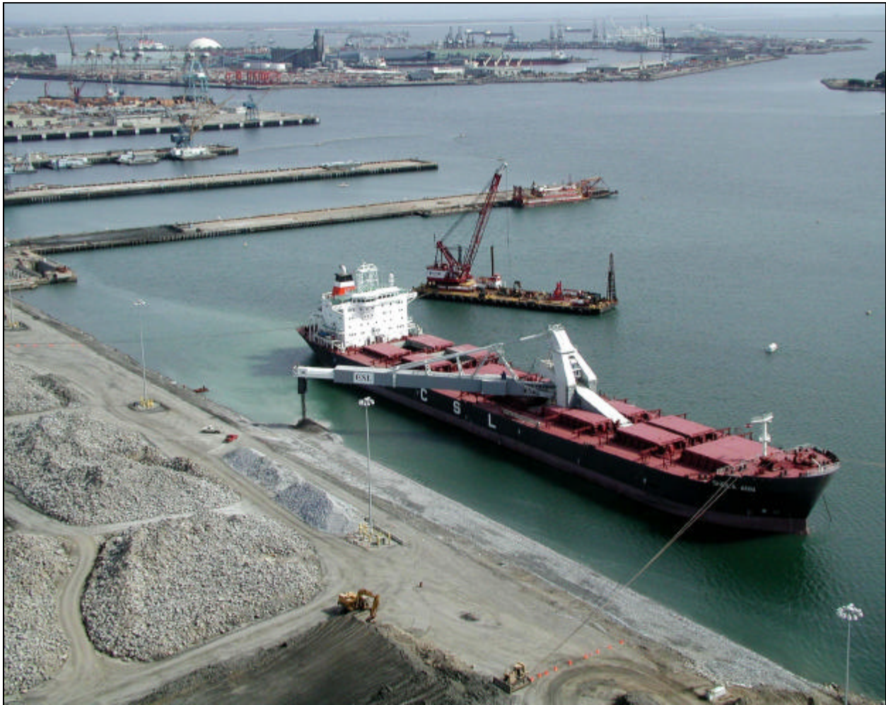
Bulk cargo deep-draft ship, the Sheila Ann, unloading aggregate at the Long Beach Harbor, Los Angeles County. Ships like the Sheila Ann can haul up to 70,000 tons of aggregate ( photo courtesy of the Port of Long Beach ).
