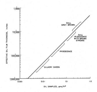
Figure 8. - Oil film appearance and effective thickness as a function of the mass of oil collected (p = 0.9 gm/cc) taken from technical memorandum 1230, General Research Corporation.
