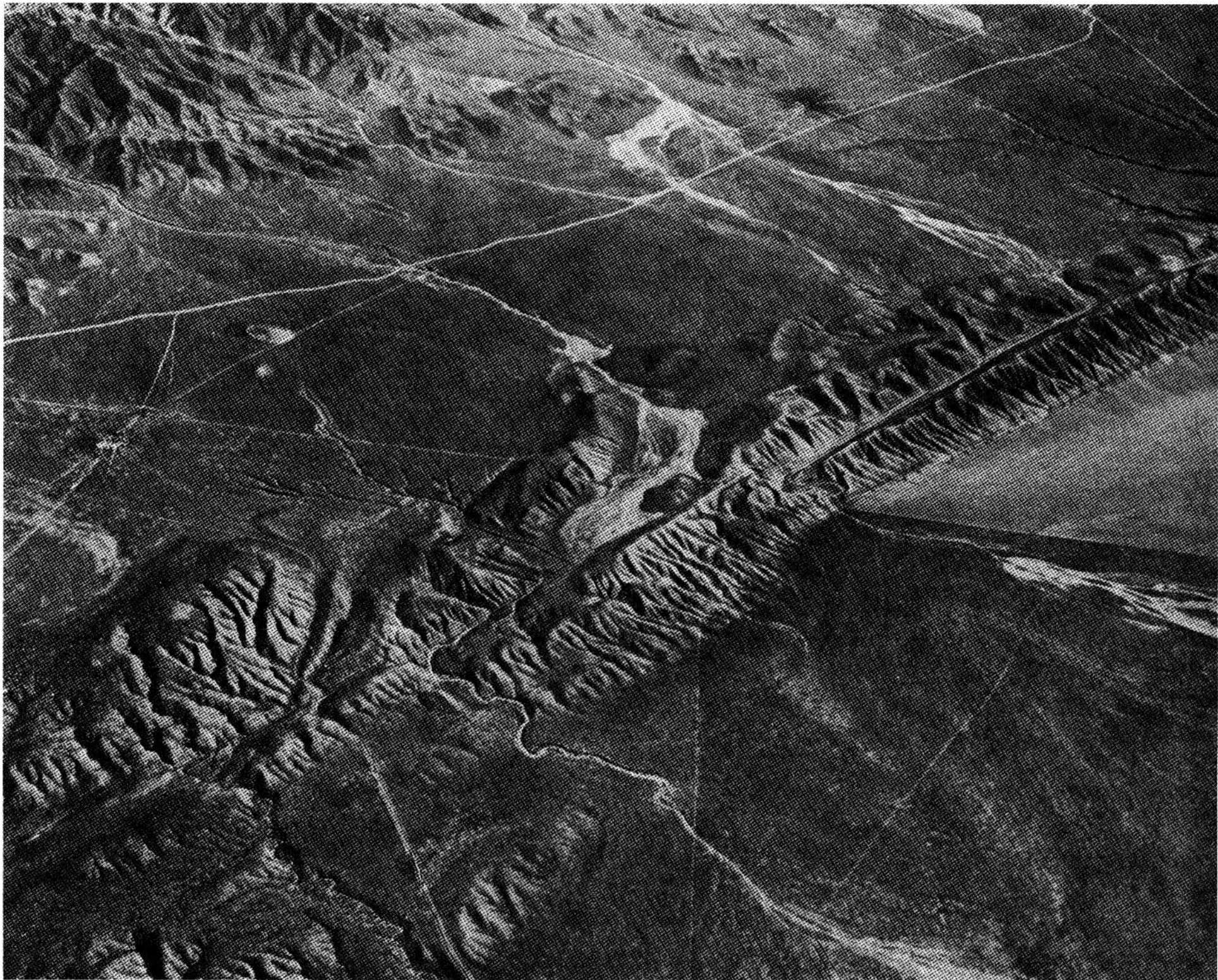
San Andreas fault in the Elkhorn Hills; view southeast from above the Carrizo Plain. A classic example of lateral fault displacement exemplified by pronounced offsets in the stream drainage where the fault slices through the Plio-Pleistocene gravels in the central part of the photo. Photo by R. C. Frampton and J. S. Shelton, 1948.
