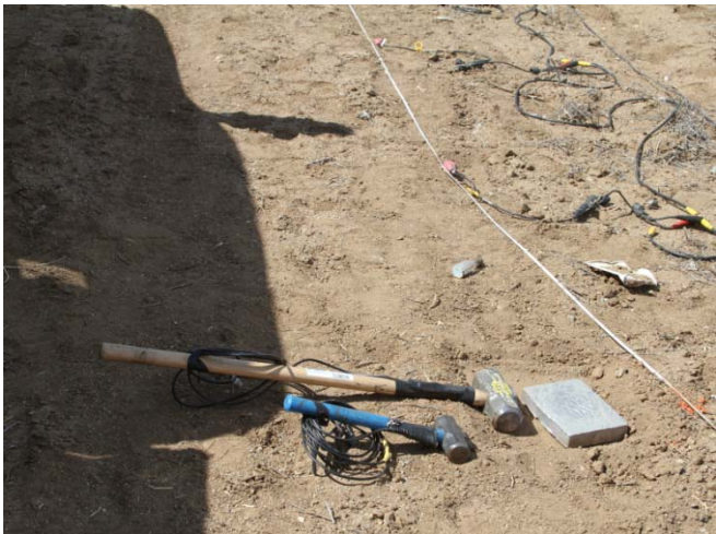
4 lb and 12 lb hammers used during data acquisition along MASW array 13924-2
