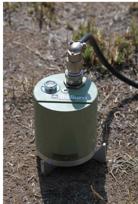
Trillium sensor used for measurements at HVSr Location 1
