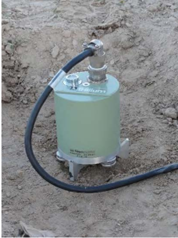
Figure 13 Nanometrics Trillium Compact seismometer used for HVSR measurements
