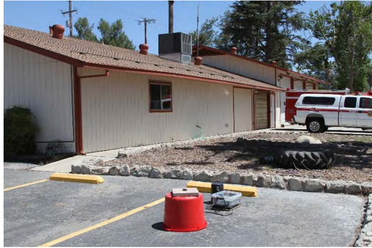
Figure 13 Nanometrics Trillium Compact seismometer used for HVSR measurements
