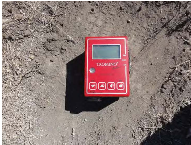
Figure 14 Micromed Tromino® ENGR seismometer used for HVSR measurements
