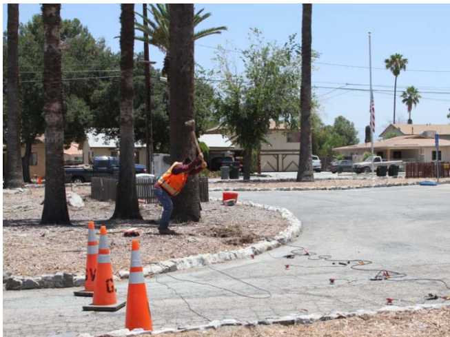
Data acquisition along MASW array 12102-1
