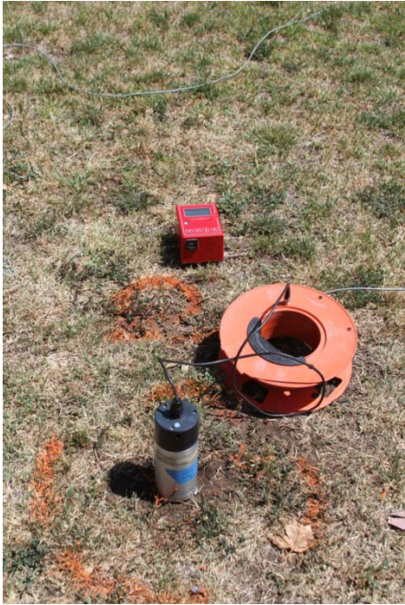
1 Hz geophone used on passive surface wave array 13925-1 and Tromino sensor used for measurements at HVSr Location 2
