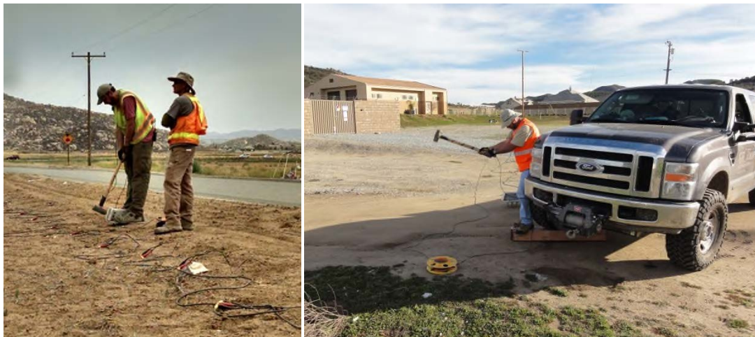
Figure 10 Hammer impact aluminum source and wood traction plank used for MAS L W acquisition
