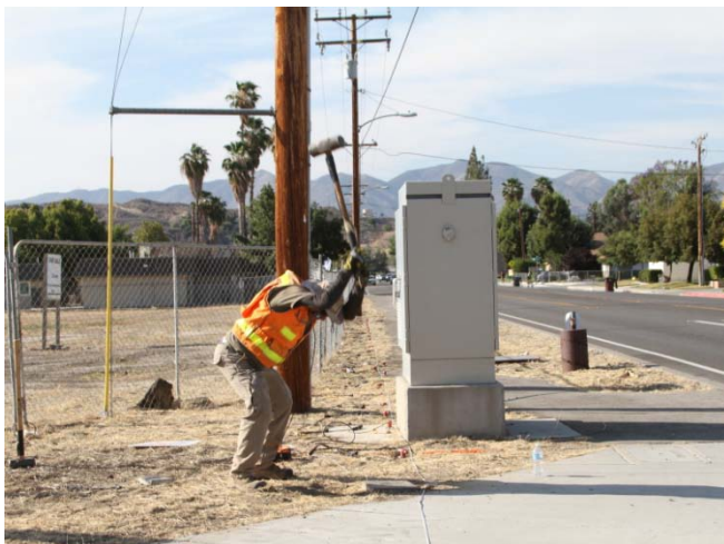
Data acquisition along MASW array 12923-2
