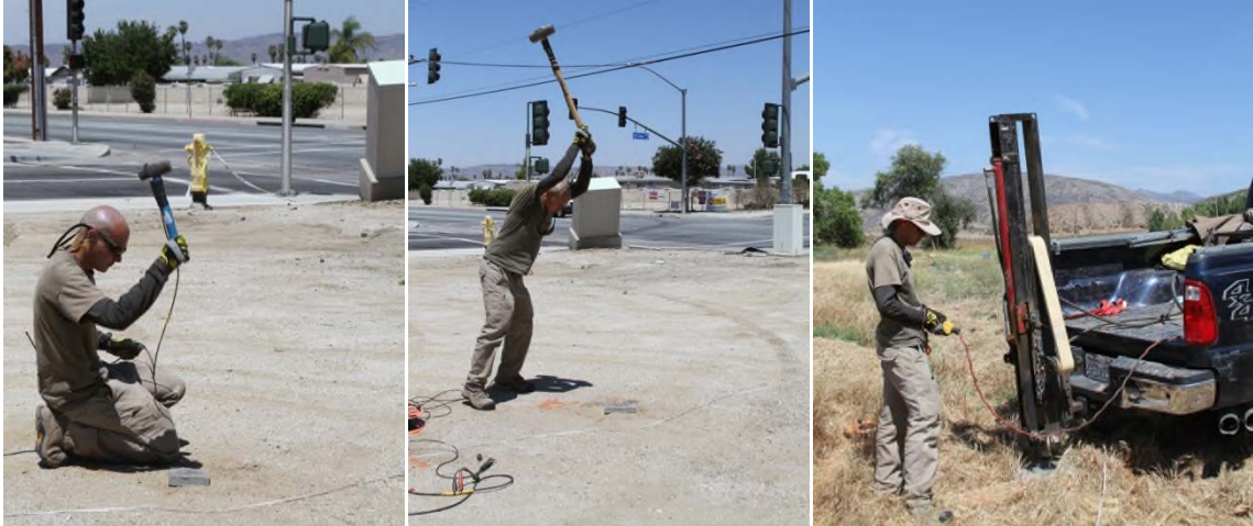
Figure 9 4 lb hammer, 12 lb sledgehammer, and 240 lb AWD used for MAS R W acquisition
