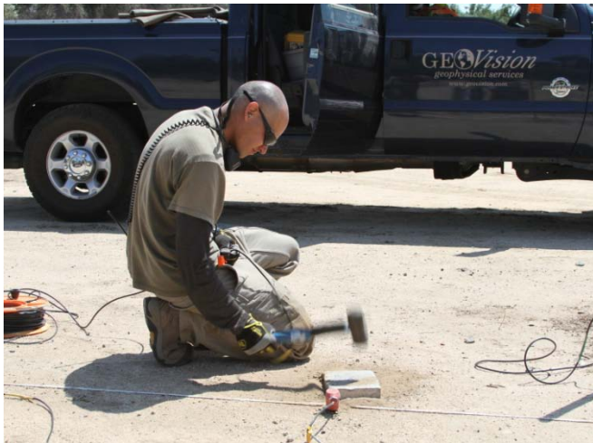
Data acquisition using 4 lb hammer on MASW array 13079-3
