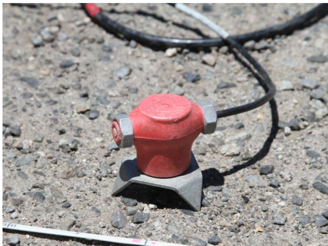
4.5 Hz vertical geophone used during MASW data acquisition
