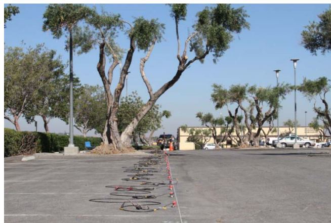
Looking west along MAS R W (Rayleigh wave) array 13123-1
