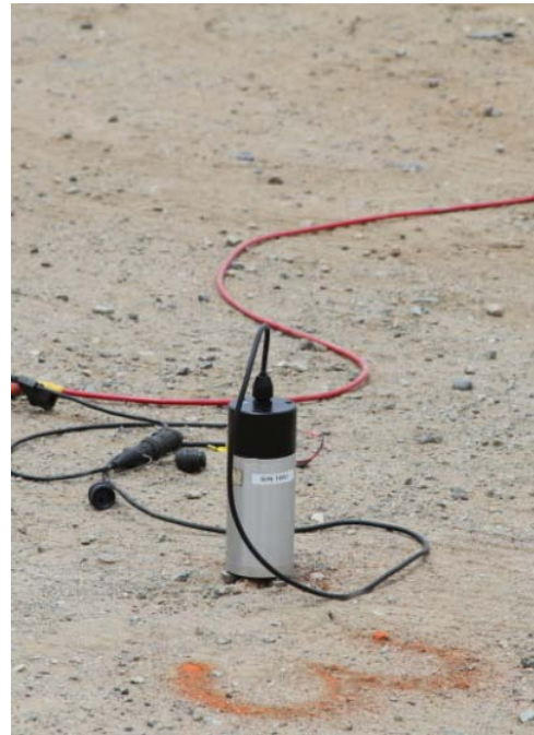
1 Hz geophone used during data acquisition along passive surface wave array 13921-2
