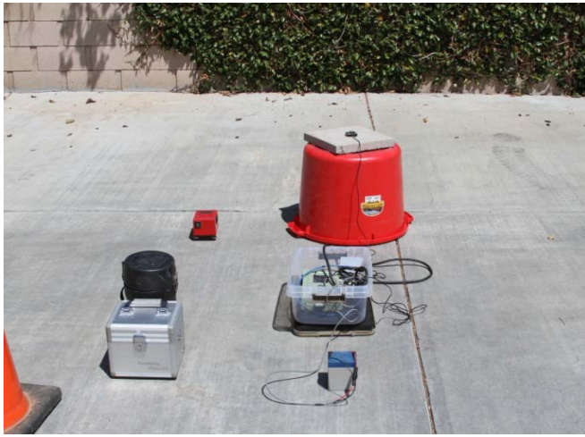
Trillium and Tromino sensors used for measurements at HVSr Location 1
