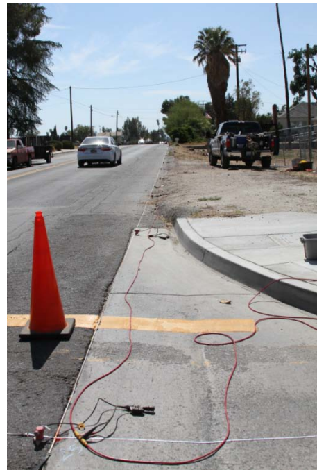
Looking west along passive surface wave array 12923-1
