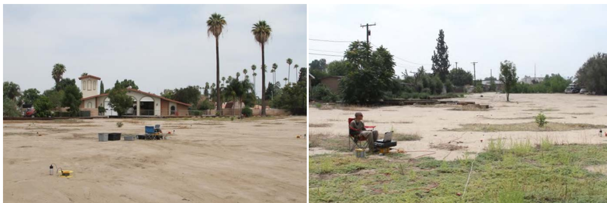
Figure 12 Nested triangle and linear arrays used for array microtremor measurements at CE.13079
