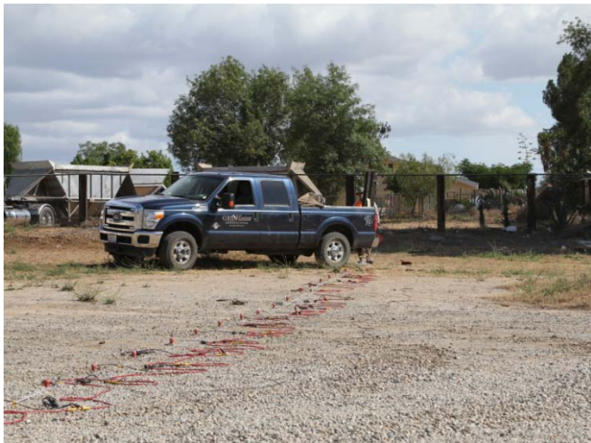
Data acquisition along MASW array 13921-3
