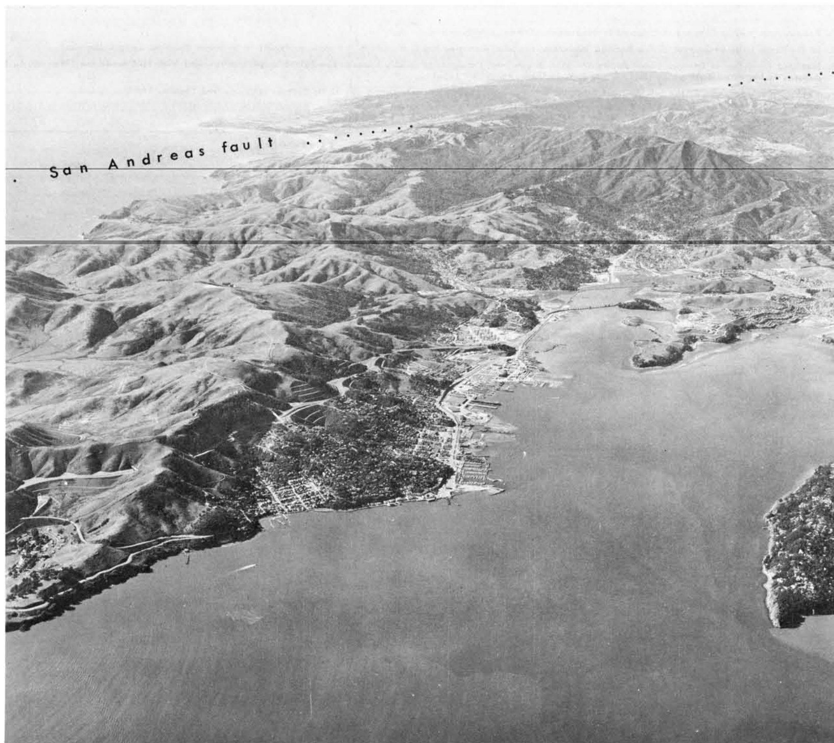
Aerial view of the Marin Peninsula northwestward toward the San Andreas fault and Point Reyes. The dissected hills in the foreground, which culminate in Mt. Tamalpais in the right middleground, are composed of graywacke, shale, radiolarian chert, greenstone, and serpentine of the Jurassic and Cretaceous Franciscan formation. The pronounced trench of the San Andreas fault separates the Franciscan formation from Mesozoic granitic rocks and Tertiary sedimentary rocks on the Point Reyes Peninsula. Photo by Aero Photographers, Sausalito.
